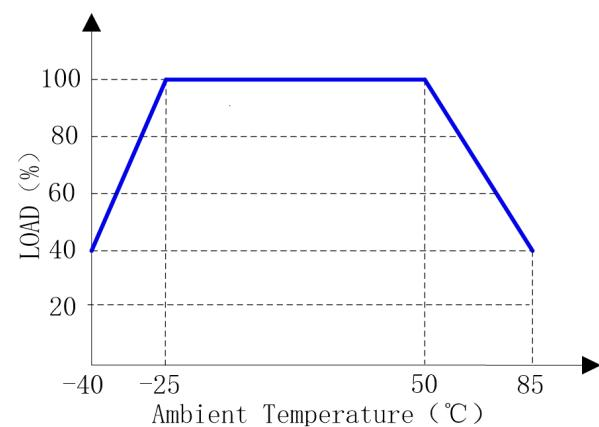
Comment: Both temperature derating and input voltage derating should be considered.
