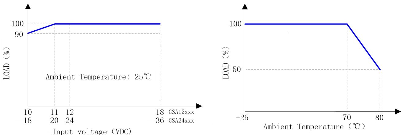
Comment: Both temperature derating and input voltage derating should be considered.
